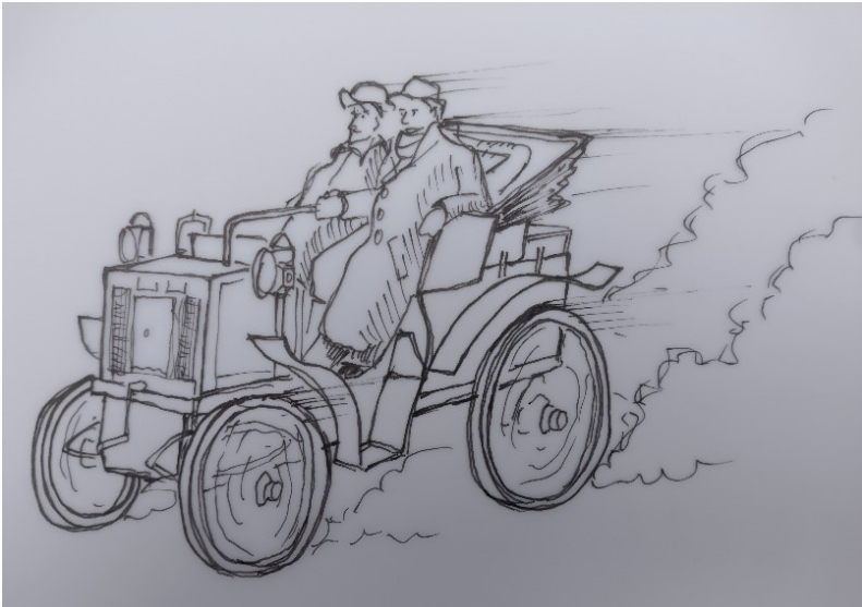
A left-hand drive, tiller steered, solid tyre 4hp P Panhard-Levassour (sketch by David Hopkins)
